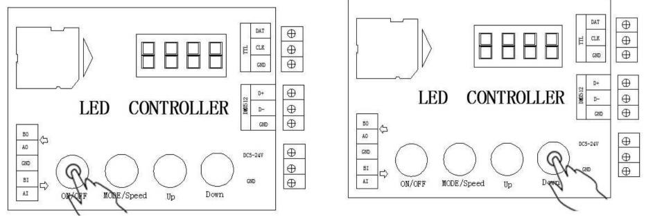
Press ON/OFF, When it display OFF, Then press UP/DOWN to setting the quantity. After doing it, Press ON/OFF to quit out.
