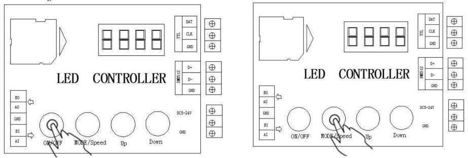
Press ON/OFF, When it display OFF, Then press MODE/Speed to choose the IC mode. After doing it, Press ON/OFF to quit out.
